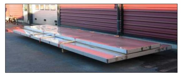
Illustration. A 7200x3600 mm-sized drying kiln door waiting for delivery to the customer.
